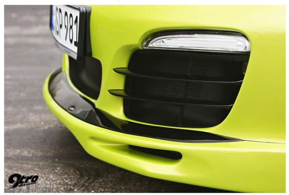
The aerodynamic additions are simple but striking. They begin with a front chin spoiler that attaches to the lower part of the front valance. Its design is a bit more radical than we are used to seeing from SpeedArt, with a distinct 'step' that is neatly highlighted by the carbon-fibre detail strip on its horizontal surface.
