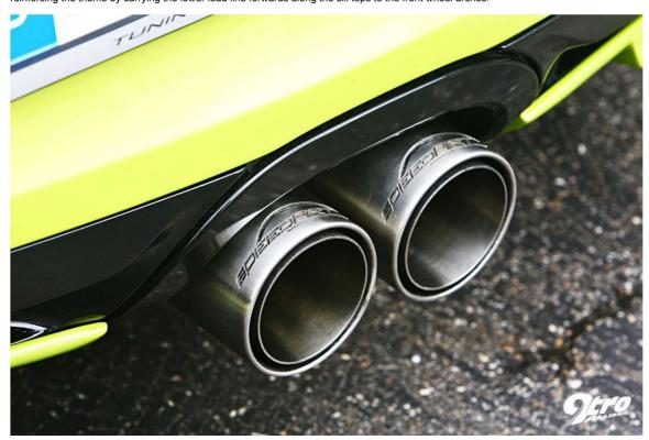
Carbon-fibre is also used for the rear valance insert, visually reducing the apparent height of the rear, and providing clear separation from the underbody diffusor. With their boundary layer fences, the two halves of the diffusor help to clean up separating air that would otherwise create drag, while flanking a pair of 98mm diameter stainless steel exhaust outlets that look like the barrels of a very big gun.
