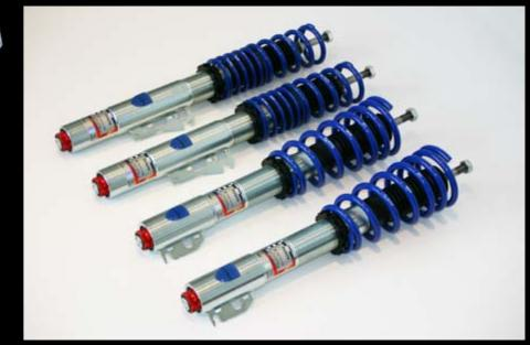
Coilover suspension setup "Race-Allround" with PASM
